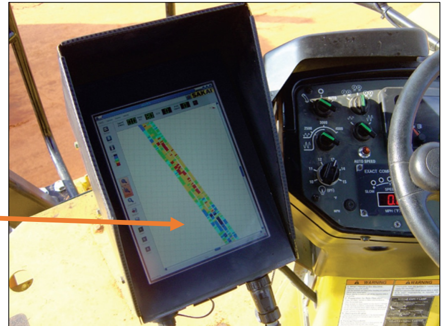
Coverage uniformity of breakdown rolling pattern.
