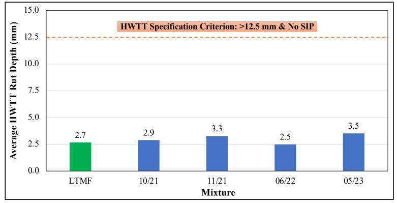
• All mixtures met the MassDOT specification criteria with all mixtures exhibiting very low rut depths and no stripping inflection point, which implies that rutting and moisture damage were not issues for these mixtures.
