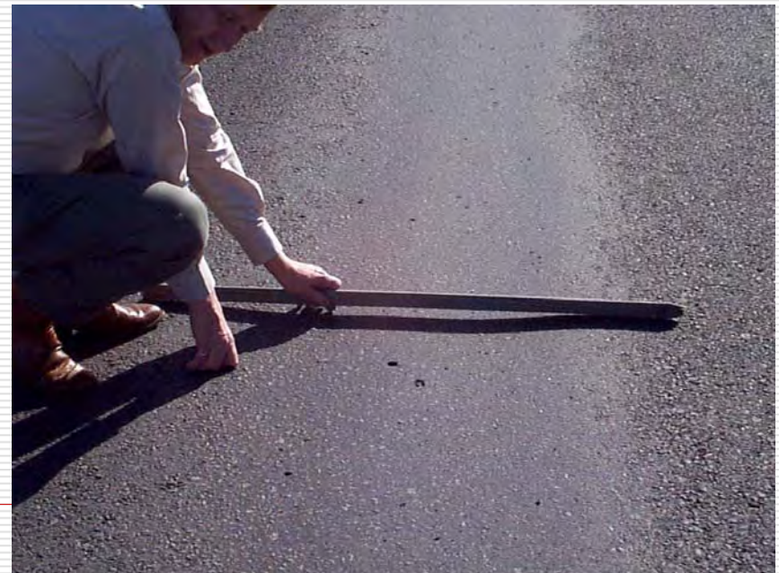
PG 67-22 unmod. 15mm rutting
