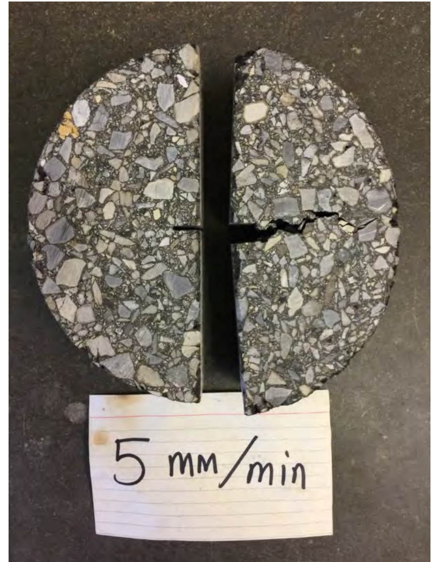
Specimens Before (L) / After (R) Testing
