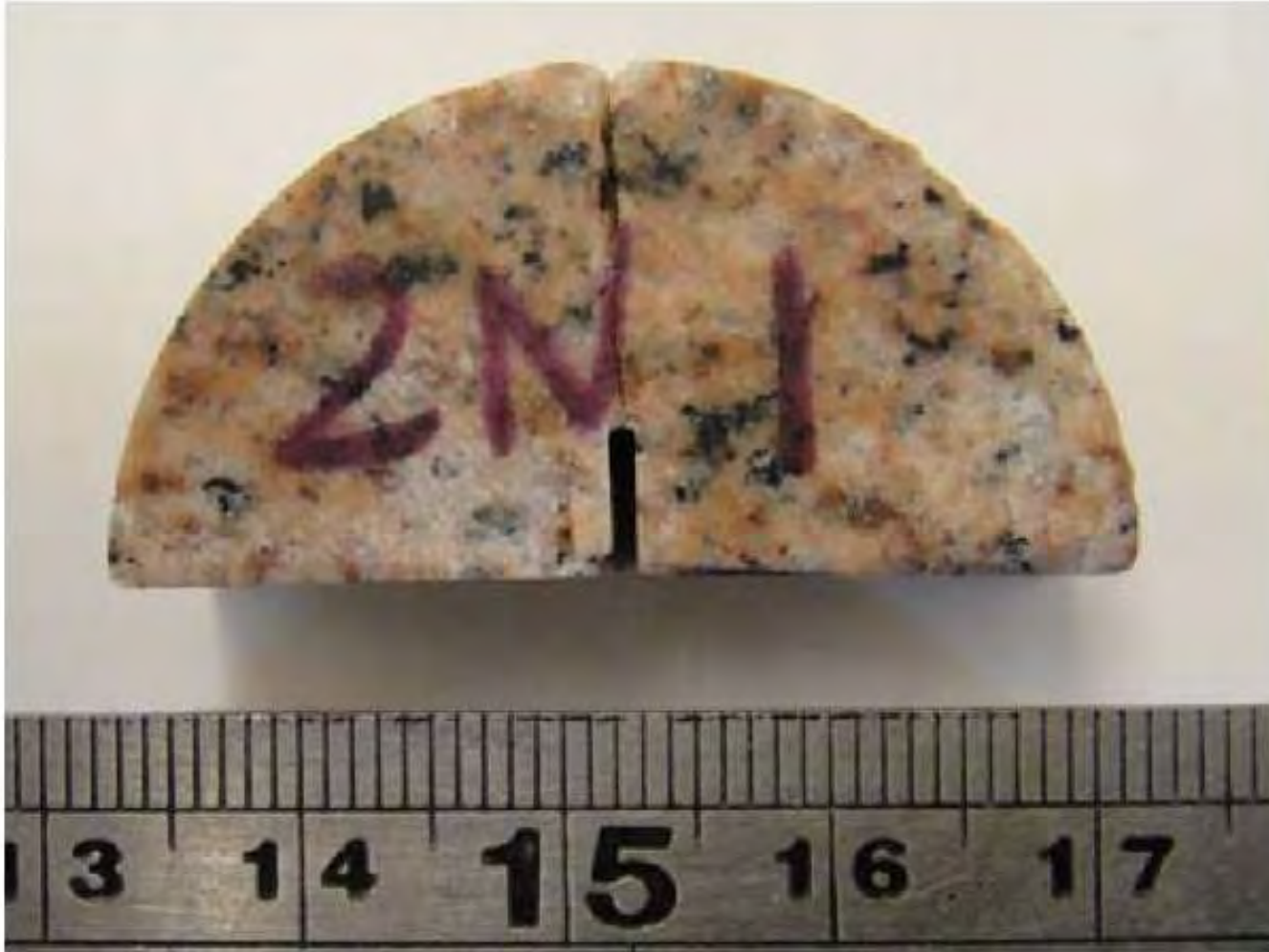
SCB Testing of Granite Rock
