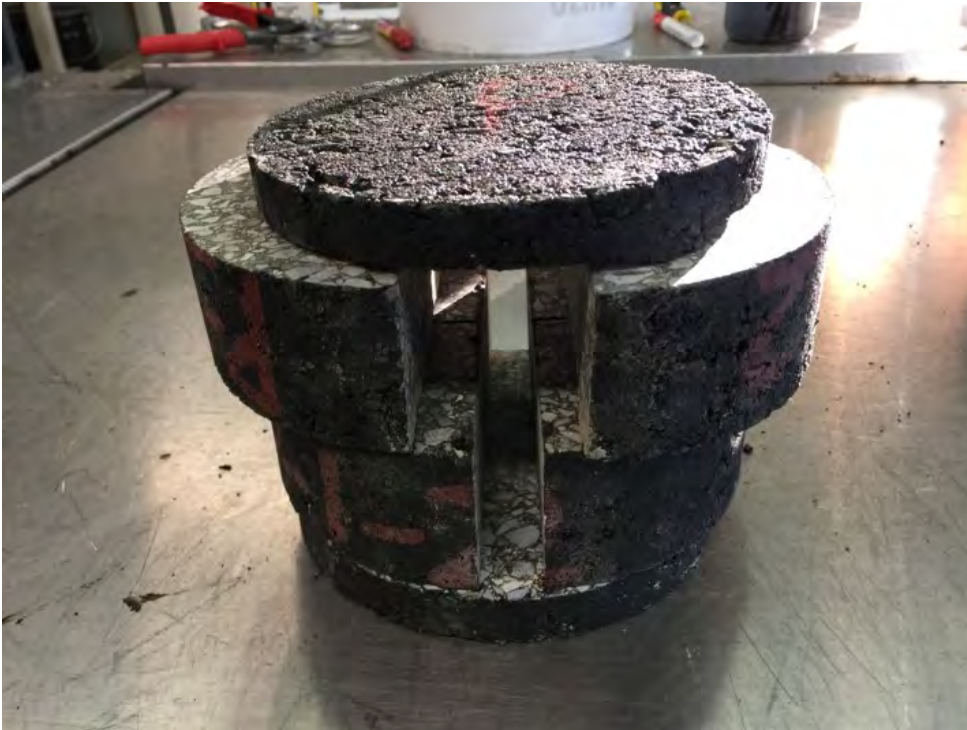
Specimens After Cutting Ready for Testing
