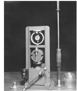
"Marshall method" pavement testing apparatus
