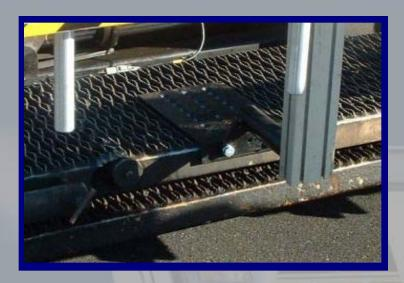
The PAVE-IR™ system mounts to the screed walkway by bolting or welding.
