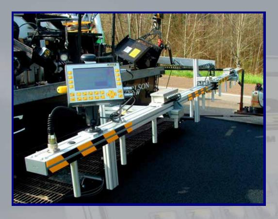
The MOBA Operand™ computer attaches to sensor beam.
