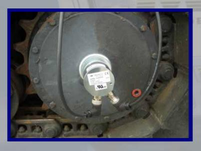
The distance encoder mounts to the wheel or torque hub using a magnet.
