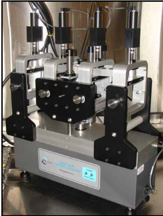
Testing in Accordance with AASHTO T321
