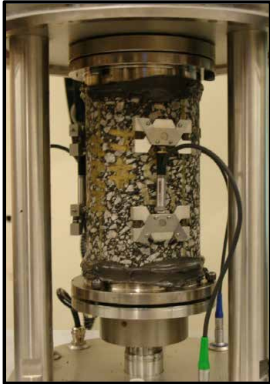
Uniaxial Cyclic Tension Fatigue (Pull-Pull)
