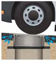
Protecting the structure below, traffic vibration is absorbed by the road surface.
