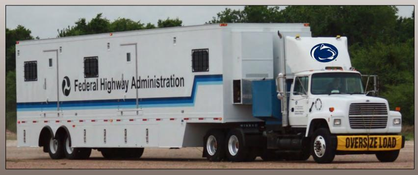
FHWA's Mobile Asphalt Testing Trailer
