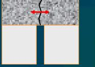
Horizontal Tensile Stress due to Expansion/Contraction of PCC from Temperature
