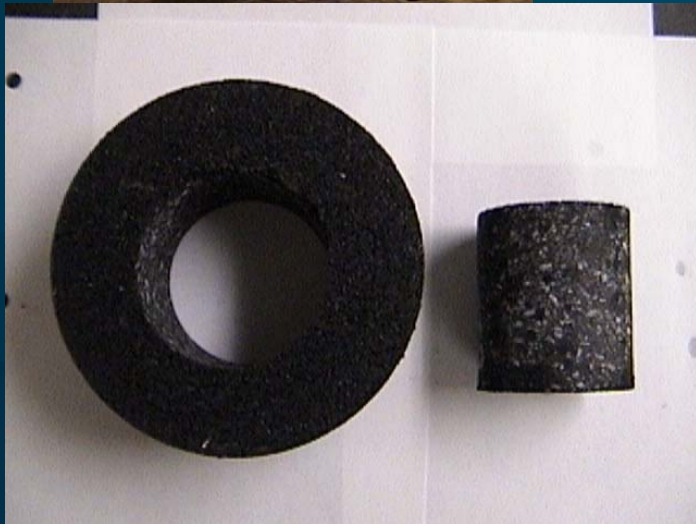
Samples cored from 6-inch diameter gyratory sample
